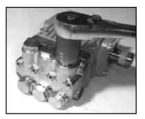
With a 22mm socket wrench, remove the (3) discharge valve plugs and (3) inlet valve plugs (32) Inspect the o-ring (33) for wear and replace if damaged.
