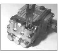
2. Using a needle nose pliers, remove the inlet and discharge valve assemblies (32X).
