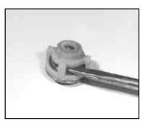
3. By inserting a small screw driver between the valve seat (27) and the valve spring retainer (30), the valve assembly can be separated.
