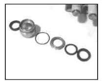
7. Remove the weep return ring (25), pressure ring (24), and v-sleeve (23) from the valve casing (26). Remove the v-sleeve (23A) from the seal case (20).
