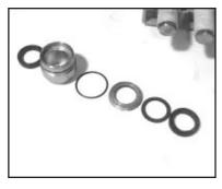
7. Remove the weep return ring (25), pressure ring (24), and v-sleeve (23) from the valve casing (26). Remove the v-sleeve (23A) from the seal case
