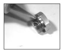
4. Remove the o-ring (31). Inspect all parts for wear and replace as necessary. Apply one drop of Loctite 243 to the valve plugs (32) and tighten to 59 ft.-lbs.
