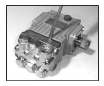
6. Carefully slide the valve casing (26) out over the plungers.
