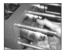
13) Pull seal sleeves (38) and plungers (36) out of their fittings in the crankcase (1) using ring groove as a guide.
