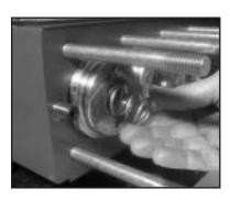
12) Remove tension spring (40) from seal retainer (38).
