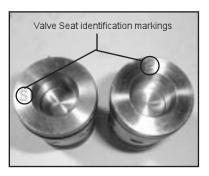
7) When reassembling: The inlet valve seat (51C) is 1mm smaller in diameter than the discharge valve seat (52C). Inlet valve seats are marked "S" and always have to be installed first. Discharge valve seats are marked "P" and are always to be installed on top of inlet valve. Plugs (58) are to be tensioned down evenly with screws (58C) and in crosswise pattern at 155 (ft.lbs.).
