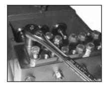
1) Lossen and remove screws (58C) with a 24mm socket wrench.
