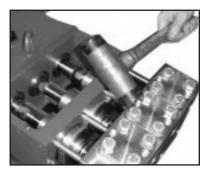
9) With a rubber mallet tap the back of the valve casing (50) and pull the valve casing off the stud bolt (49).
