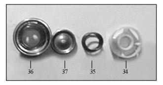
If pitted or worn, replace inlet valve seats (36), valve plates (37), springs (35) and spring retainers (34). Reinsert items 34-38 into valve adapter (39). Install valve assembly (34-40) into manifold (29). Reinstall manifold plugs (43) and torque plugs to 50 ft.-lbs.
