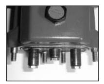
14. Before replacing pump manifold (29), first rotate crankshaft (18) until two outside plungers (24A) extend evenly forward. Next lubricate v-sleeves (50) in the rear v-sleeve housing (48) and slide housing over plungers. Lubricate ceramic plungers with a light film of oil. Carefully and evenly slide manifold over plungers and press manifold firmly against crankcase (1). Replace manifold stud bolts (45), washers (47) and nut (46) and tighten to 35 ft.-lbs.
