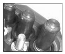
11. Inspect ceramic plunger (24A) tips for wear. If necessary, replacement of the ceramic plungers may be accomplished by removing the plunger bolt assemblies (24B and 24C) with a 13mmwrench. Ceramic plungers should now slide off the stainless steel plunger base (22). Excessive resistance to plunger removal may be overcome by heating the stainless steel plunger base. This will melt any excess loc-tite beneath the ceramic plunger allowing easy removal.
