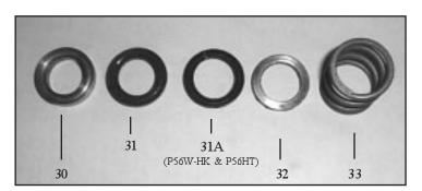
8. Inspect and clean the manifold and pressure ring. Reinstall the pressure ring (30) with the groved side pointed towards the front. Insert v-sleeve (31) high temperature seals (31A for P56W-HK &P56HT pumps), support ring (32), and pressure spring (33) into the manifold (29).
