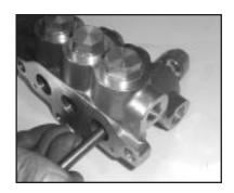
From the front inlet valve ports, remove the inlet valve assembly (34-40) and pressure springs (33).
