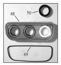
10. The rear v-sleeve housing (48) may be removed by prying evenly outward with a flat screwdriver. After slipping housing over ceramic plunger (24A), inspect seals (50) and o-ring (49) and replace as necessary. If the crankcase is to be disassembled, the housing should not be replaced until later.
