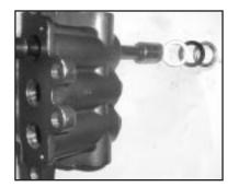
Turn the manifold (29) over. Using a 15mm socket, tap out the v-sleeves, Insert v-sleeve (31) high temperature seals (31A for P56W-HK &P56HT pumps), support rings (32), and pressure rings (30) through back of manifold.
