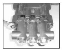
4. Drain the oil from the pump. Turn the pump over to remove the four manifold stud nuts (46) with a 17mm wrench.
