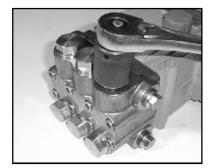
1) With a socket wrench, remove the three discharge valve plugs and three inlet valve plugs (32). Inspect the o-ring (33) for wear and replace if damaged.
