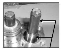
9) Check surfaces of plunger pipe (16B).
