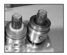
10) Place each seal case (20) with new o-rings (21 and 22) and new oil seals (19) over plungers (16) with weep hole down. Generously lubricate o-rings and oil seals before reassembly.
