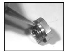
4) Remove the o-ring (31). Inspect all parts for wear and replace as necessary. Apply one drop of loctite 243 to the valve plugs (32) and tighten to 125 ft. lbs.
