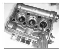
7) Remove the pressure rings (24), and v-sleeves (23) and spacer ring (23A) from the valve casing (26). Remove the remaining v-sleeves (23B) and pressure rings (24) from the seal case (20).
