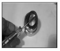
8) Remove the weep grooved seal (23 or 23B) together with pressure ring (24 \_ P420 and P425 only) out of the seal adaptor (20). Check O-rings (21).
