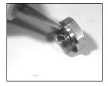
Remove the o-ring (31). Inspect all parts for wear and replace as necessary. Apply one drop of Loctite 243 to the valve plugs (32) and tighten to 59 ft.-lbs.
