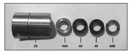
11) Remove the pressure ring (40A), v-sleeves (40), and support ring (40B), from the seal sleeve. Remove the pressure spring (41). Examine seals carefully and replace if worn. Clean surfaces of seal sleeves (35) which come in contact with the crankcase (1) and sealing surfaces of valve casing (43).
