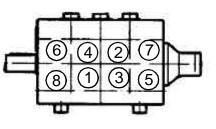
15) Tighten hex nuts (49A) in a crosswise pattern (shown above) to 59 ft.-lbs.
