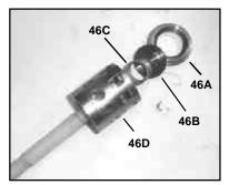
4) Loosen valve seats (46A) and valve spring (46C) from spacer pipe (46D) by lightly hitting the valve plate (46B) with a plastic stick. Check sealing surface and replace worn parts. Reassemble with new orings (44A) if possible and oil them before installing.
