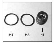
2) Remove the support ring (44B), o-ring (44A) and tension spring (45).
