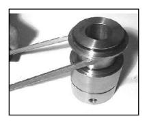
9) Remove seal case (37) from seal sleeve (35).
