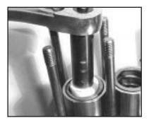
11. Tighten the tension screws (29C) to 310 in.-lbs. The plunger pipe (29B) should not be strained by over tightening of the tension screw (29C) or through damage to the front surface of the plunger; otherwise, it will probably break.
