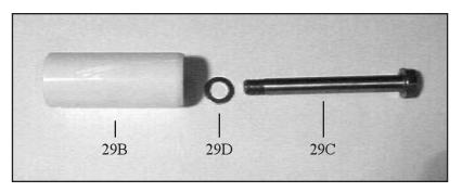
9. Check plunger surface (29B). If plunger pipe is worn out, loosen tension screws (29C) and pull off plunger pipe to the front. Clean front surface of plunger (25) thoroughly. Apply a thin coat of Loctite to the tension screw threads (29C). Note: Care must be taken that no glue gets between the plunger pipe (29B) and the centering sleeve (29A). Add new copper ring (29D).
