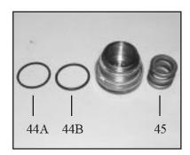
2. Remove the compression spring (45) & o-rings (44A & 44B-LP250W-MT only).
