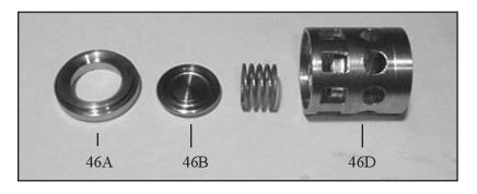
4. Loosen valve seats (46A) from spacer pipe (46D) by lightly hitting the valve plate (46B) with a plastic stick. Check sealing surface and replace worn parts. Reassemble with new o-rings (44A) if possible and oil them before installing. Tighten up tension plugs (48) to 107 ft.-lbs.
