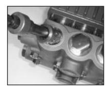
3. Remove the complete valve assembly (46) with valve pullers.
