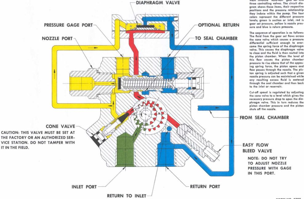
The A-70 has a unique circuit that exhibits a dependable cut-off, a high single pipe lift capacity and automatic two pipe purging.
