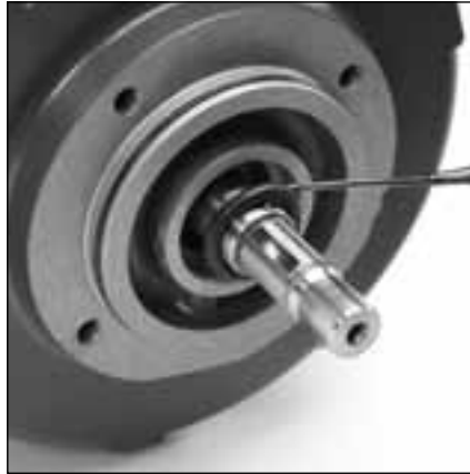
5.9 Remove and inspect slinger o-ring (11) from motor flange.
