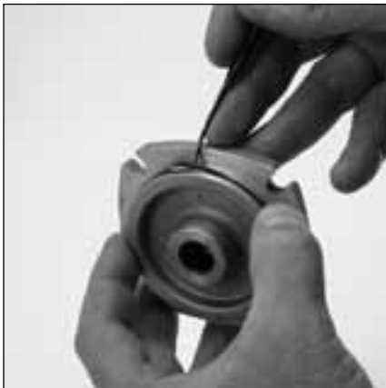
6.7 Lubricate and install o-ring (6) onto bearing cover (5).
