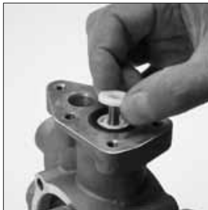
6.17 Install inlet valve (20) with flat side down onto plunger (21).
