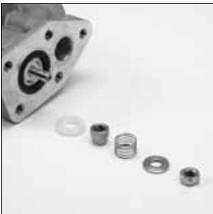
5.14 Remove and inspect nut (16), washer (17), spacer (19), spring (18) and inlet valve (20).
