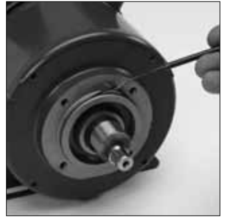
6.3 Lubricate and install o-ring (12) onto motor flange.
