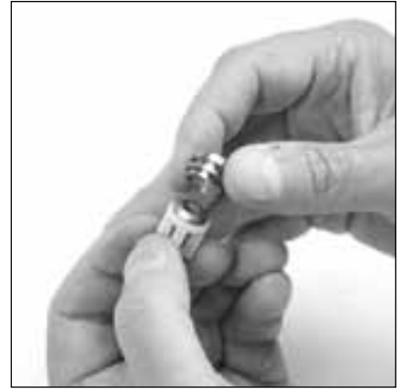
6.12 Place tapered side of seat (24) towards retainer (27) and snap into place.
