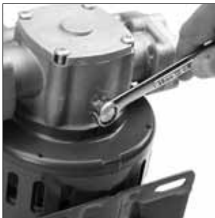
5.2 Remove brass drain plug (3) from pump crankcase (1) to drain water.
