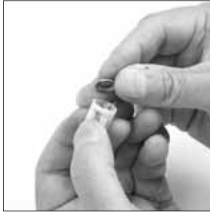
6.11 Place valve (25) cupped side over the spring (26).
