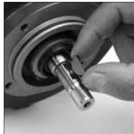
5.7 Remove and inspect woodruff key (9) from keyway of motor shaft.
