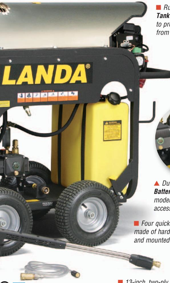
■ Rust-free, 10 gal. **Fuel Tank** with elevated fuel line to prevent dirt and debris from reaching burner.
