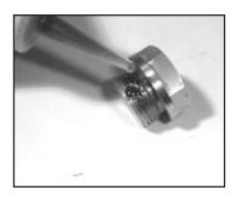
4. Remove the o-ring (31). Inspect all parts for wear and replace as necessary. For pumps manufactured prior to 5/97, tighten plugs (32) to 33 ft-lbs. otherwise, apply one drop of Loctite 243 to the valve plugs (32) and tighten to 59 ft.-lbs.
