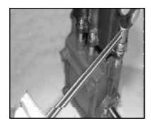
39. Again lubricate the plungers (29B) and slide the manifold (#43) gently and evenly over the plungers. Press the manifold firmly into place against the crankcase (#1). Install the spring washer (#50A) and tighten the manifold stud nuts (#50) to 58 ft.lbs.
