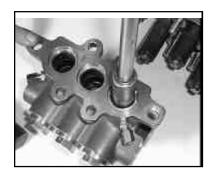
6. To remove the inlet valve assembly, insert a 13mm socket with extension through the rear of the inlet manifold (#43) port and tap it firmly with a hammer. This will force the tension spring (#46), valve housing (#52) and the remainder of the inlet valve assembly out through the front of the inlet port.
