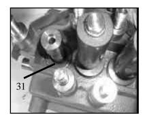
11a. Inspect the crankcase oil seals (#31) for evidence of leaking. If there is oil on the crankcase (#1) at the sight of the oil seals, they must be replaced. The oil seals are replaced after removing the crosshead/plunger assembly (#25) as described below.
