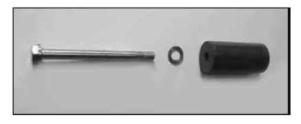
11. To remove the ceramic plungers, turn the plunger bolt (#29C) counterclockwise with a 13mm socket. Use a steady torque to prevent ceramic plunger sleeve damage. Loosen and remove the plunger bolt assembly (#29C and #29D) and replace the seal washer (#29D).
