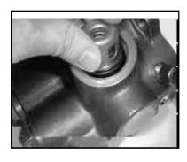
37. Place the entire discharge assembly into discharge port making certain the assembly is properly seated. Install discharge plug (#48) and hand tighten.
