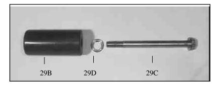
32. Inspect the ceramic plungers (#29B) and replace them if necessary. Clean the ends of the ceramic and remount onto the crosshead/plunger assembly. Make certain that the end of the plunger which is not counter-bored is facing the discharge side of the pump. Install the seal washer (#29D) on the bolt assembly.
