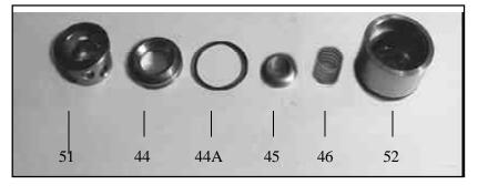
7. Pull the inlet valve assembly apart for inspection. Any resistance may be overcome by placing the valve housing (#52) in a brass jawed vise and carefully tapping the back of the valve plate (#45) with a screwdriver. Remove the spacer pipe (#51) valve seats (#44), o-ring (#44A), valve plate (#45), spring (#46), replace them as necessary.
