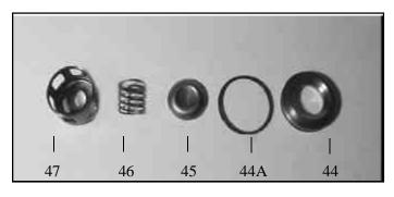
4. Inspect all parts, especially the seating surface of the valve plate (#45), and replace as necessary.
