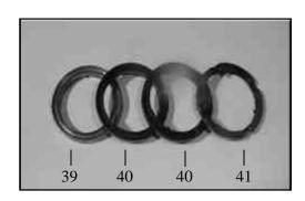
35. Reinstall the pressure ring (#39), v-sleeves (#40) and support ring (#41) into each plunger bore. Reinstall the tension spring (#42).
