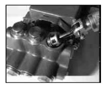
3. Using a valve puller (available from Snap-On-Tools), remove the valve assembly (#44 - #47).
