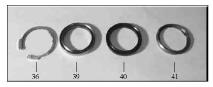
9. Turn the manifold (#43) over and remove the rear v-sleeve snap ring (#36). Remove rear pressure ring (#39), rear v-sleeve (#40) and rear support ring (#41). These parts should slide out with little resistance. If necessary, a screwdriver may be used to pry outward. Replace all rubber parts and inspect the metal parts for wear.
