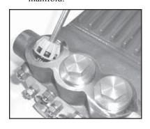
17. Next, place valve assemblies (46A) into manifold after first lubricating the o-ring (44A). Seat firmly into manifold.
