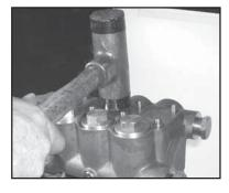
15. Place entire manifold/seal sleeve assembly over the studs and push firmly until seated against the crankcase.
