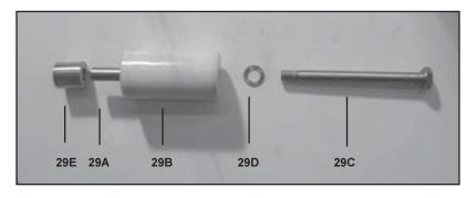
6. Inspect surface of plunger pipe (29B) carefully. Remove any chemical or mineral deposits taking care not to damage the surface of the plunger. If plunger pipe is worn, remove the plunger bolt (29C), plunger pipe (29B) and spacer (29E). Replace worn parts necessary. Note: Always use a new copper gasket (29) when repairing the plunger assembly.
