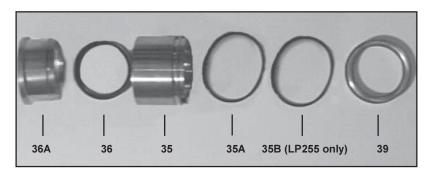
12. Lubricate weep seal (36). Place, weep seal (36), and pressure ring (36A) into the seal sleeve (35). Assemble the o-ring (35A and 35B for LP255 only) onto seal sleeve and lubricate.
