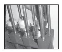
10. For LP122A & LP122A-4000 pumps, generously lubricate the inside of the oil seals (31A & 33) and o-ring (32A). Next, place the seal retainer, complete (31) over the steel plunger base seat firmly into the crankcase. Replace the flinger (30).
