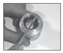
3. The back-up seal (33) can be pried out of the back of the retainer (32) with a small screwdriver. To replace with new seal, lubricate edges of new seal, then squeeze outside edges of seal, forcing the seal to collapse into a figure 8. Tuck the two outside edges of the figure 8 into the rear of the retainer, making sure that the inner lip of the seal faces the oil. The seal may now be pressed firmly into place.
