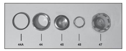
2. To disassemble the valve, screw the bolt into the retainer until the valve plate (45) presses the valve seat (44) out of the spring retainer. Examine all parts and replace if necessary. If the seat doesn't come out, use a valve puller to remove.
