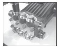
18. Replace plug with o-ring (48, & 48A) and tighten to 160 ft.-lbs.
