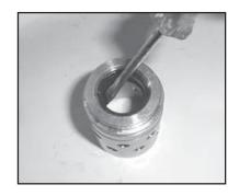
The front oil seal (31A) can now be removed by inserting a screwdriver through the rear of the retainer and tapping the seal out through the front of the retainer. Remove any excess old loc-tite from retainer. To replace oil seal, apply a light film of loc-tite around outside edges of seal. Tap seal firmly into the retainer with a wooden dowel making certain that the spring side of the seal is installed first and that the seal sits squarely in the retainer.
