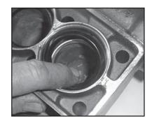
13. For LP255 pumps, insert support ring (37) into valve casing (43). Place support ring (41) and v-sleeves (40) into valve casing.
