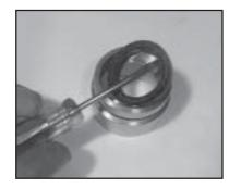
8) Remove the weep grooved seal (23B) together with pressure ring (24) out of the seal case (20). Check O-rings (21). **IMPORTANT!** The grooved seal (23) on the high-pressure side is to be fitted carefully into the valve casing (26) using a screwdriver. Under no circumstances must the seal surface in the valve casing or the seal lip be damaged.
