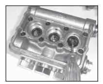
Remove the pressure rings (24) and grooved seals (23) from the valve casing (26).
