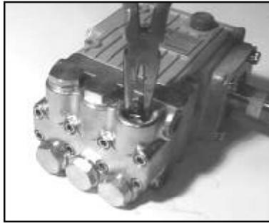
2. Using a needle nose pliers, remove the inlet and discharge valve assemblies (27-31).
