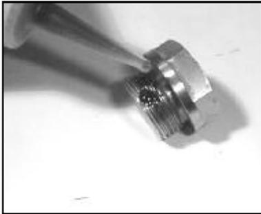
4. Remove the o-ring (31). Inspect all parts for wear and replace as necessary. For pumps manufactured prior to 5/97, tighten plugs (32) to 33 ft-lbs. otherwise, apply one drop of Loctite 243 to the valve plugs (32) and tighten to 59 ft.-lbs.
