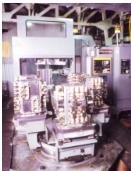
CAT PUMPS are manufactured using advanced methods to assure a well made, quality pump. Computer controlled machining centers assure quality and accuracy during pump manufacturing.
