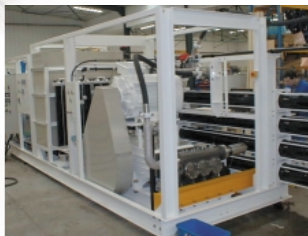
150 Frame Salt Water Reverse Osmosis Systems
