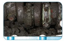
• Oil viscosity change shown causing loss of oil lubricity leading to component discoloration and failure
