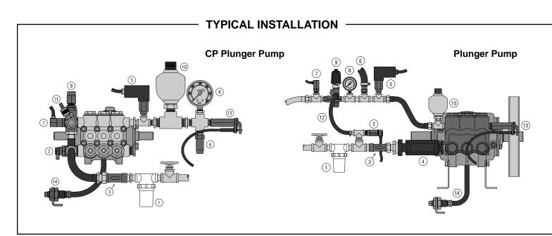
It is recommended that a secondary protective device such as the *CAT PUMP Pop-Off Valve* be installed to assure pump protection should the regulator malfunction. Refer to Troubleshooting for more information on malfunction of regulator.
